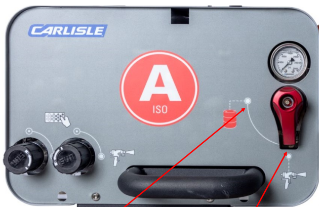
Output to drum or container from recirculation line.
