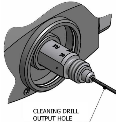
Cleaning "Round" Chamber Product Output Hole
