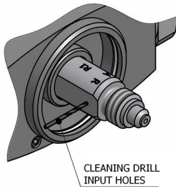
Cleaning "Round" Chamber Product Input Holes
